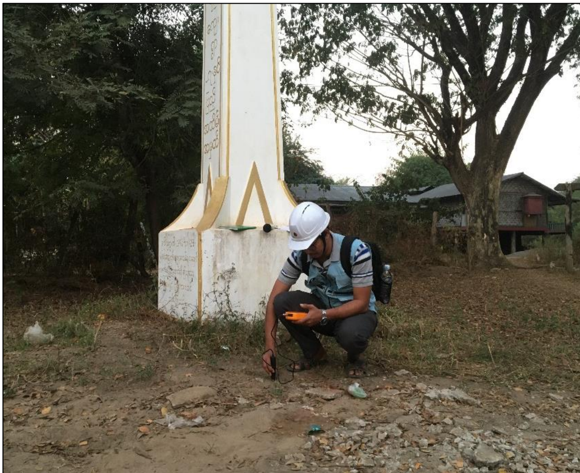
Figure 2-18 Vibration measurement in the field
