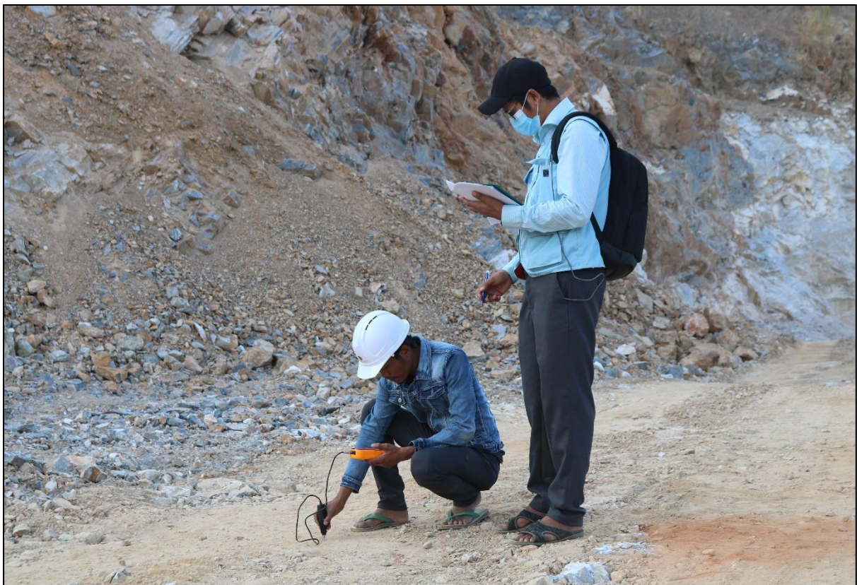
Figure 1-14 Vibration measurement at Mining Site
